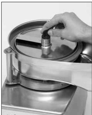
Next fit the appropriate slicing disc and screw the slicer on the motor shaft with the butterfly nut.
