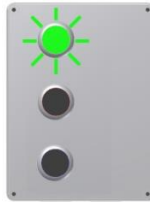
Flashing Green Machine Stopping
